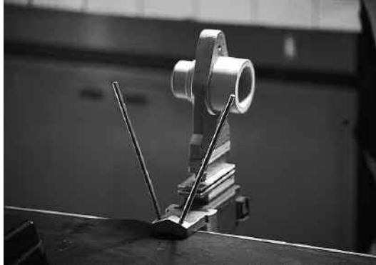
Photo 1: Appliance for manual joining of pipes and fittings by socket welding
